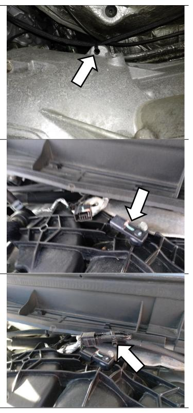
Install supplied zip-ties to support the wiring harness.
