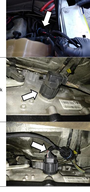
Install supplied zip-ties to support the wiring harness between the engine bay and transmission.
